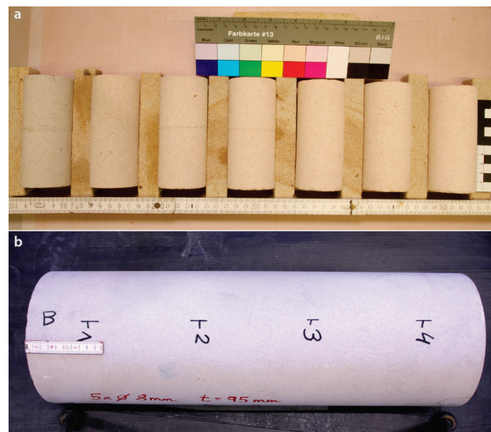
Fig. 2.1: Investigated specimens of Posta type Elbe sandstone: a) small cylinders (50 mm x 100 mm) b) large cylinder (19 cm x 58 cm).
