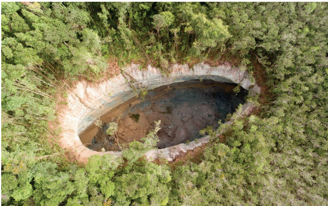
Figure 5: Sinkhole over the edge of a cavern field in a depth of more than 1000 m (Photo: OrthoPixel).
